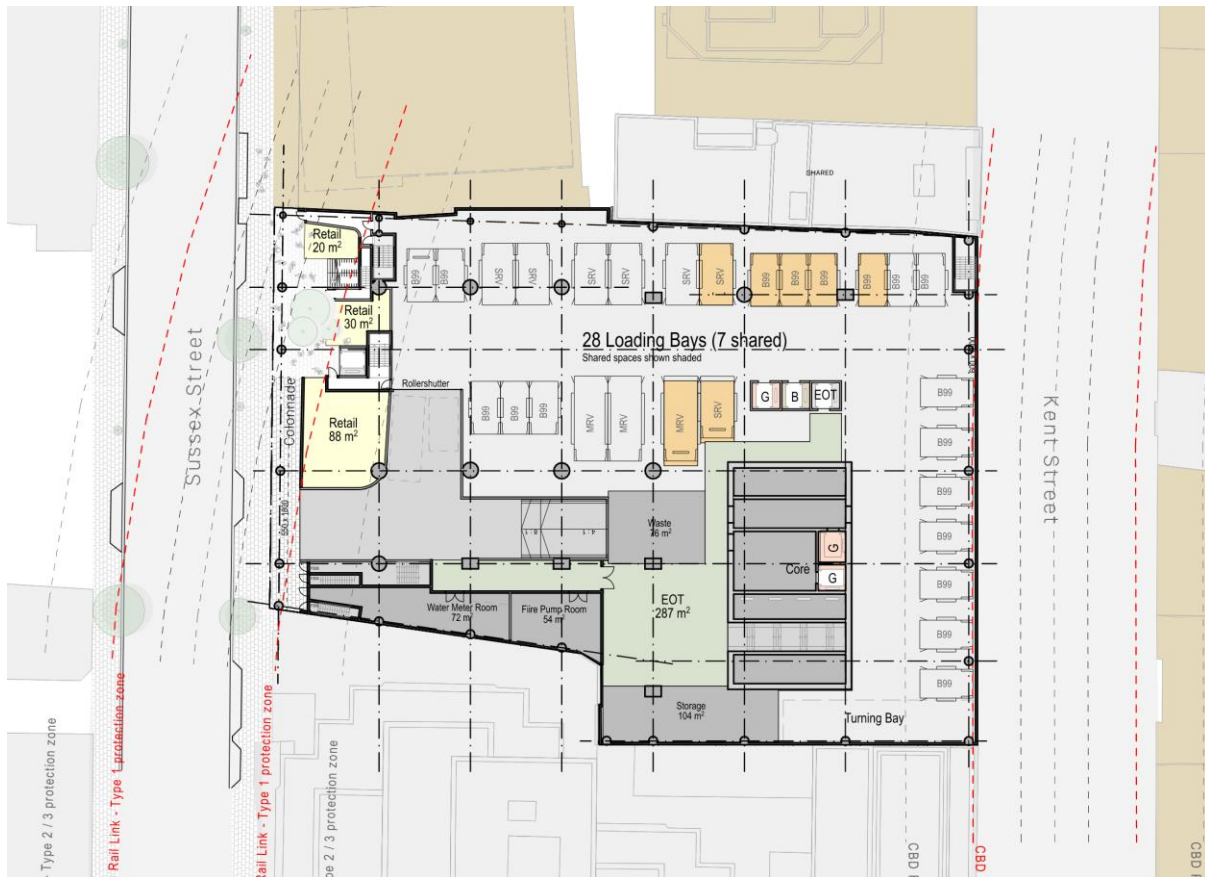
Figure 19: Sussex Street loading dock
